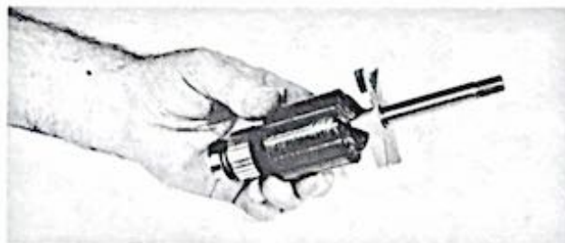
Figure 1-19. Bent armature ventilating fan blades
