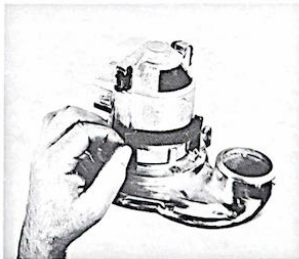
Figure 1-53. Installing vent rubber on motor housing.
