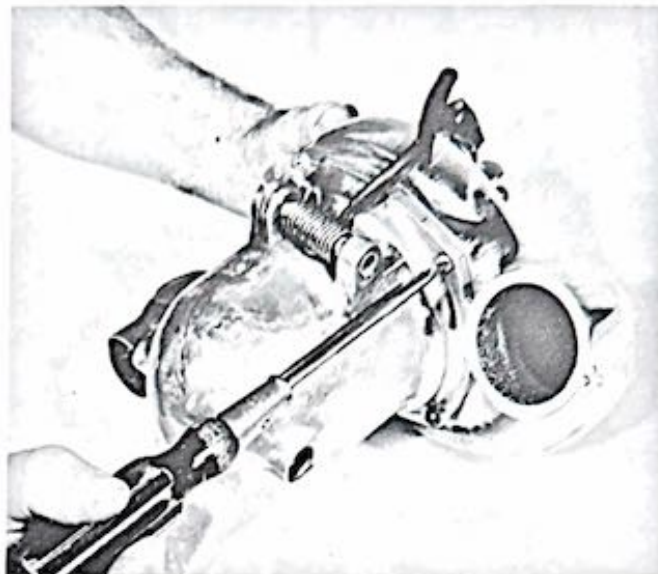
Figure 1-13. Removing fan housing screws
