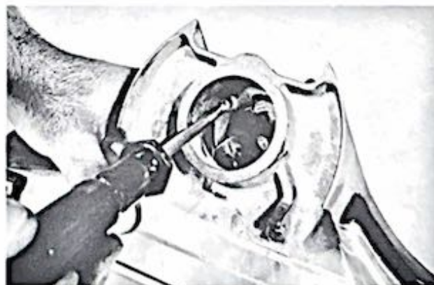
Figure 2-7. Removing belt lifter stop screw
