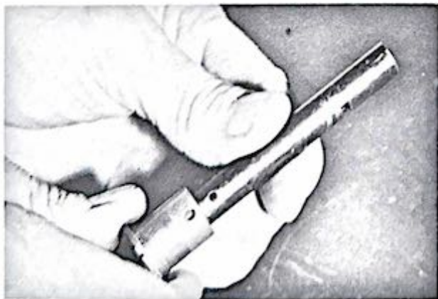
Figure 1-61. Installing bushing on spring shaft
