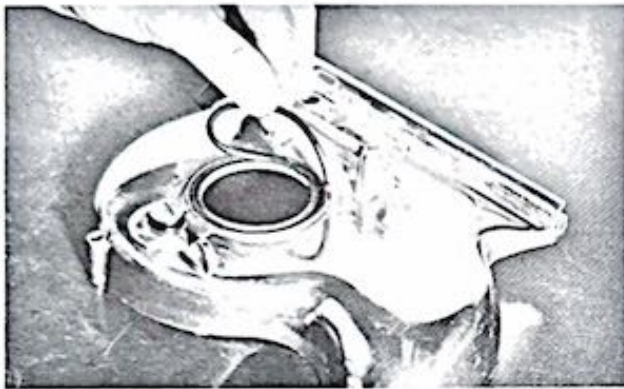
Figure 1-57. Installing seal O-ring on fan housing
