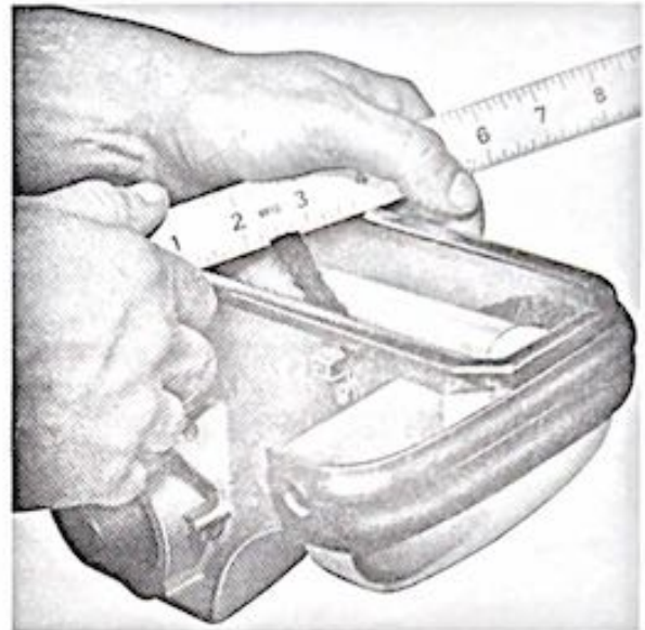
Figure 20. Checking nozzle brush protrusion
