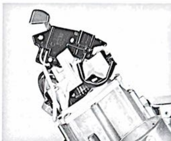
Figure 1-4. Positioning the foot switch in motor bell housing
