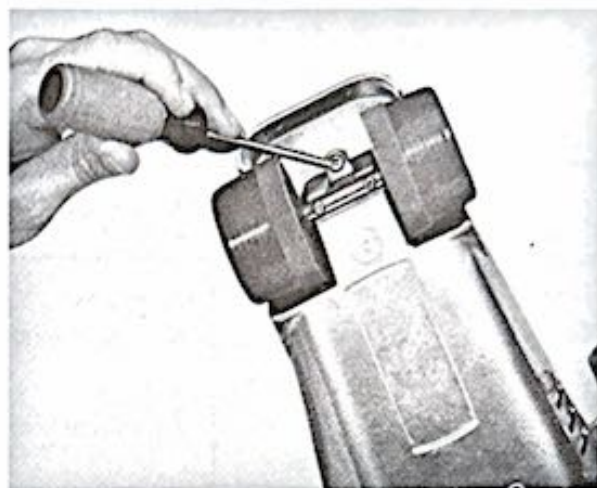
Figure 1-3. Loosening bottom foot switch screw
