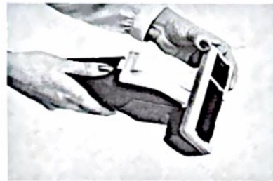
Remove base plate by sliding bottom latch back and belt cover by removing screw. Next, remove belt from pulley (may help to turn brush backwards slightly). Pull belt and brush assembly out and replace belt. Before replacing base plate and belt cover, make sure
