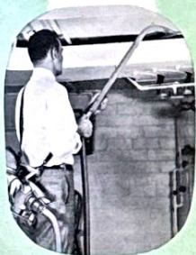
SHOULDER PORTABLE Add the shoulder strap to the floor portable and you have a unit which frees both hands for work in difficult places.
