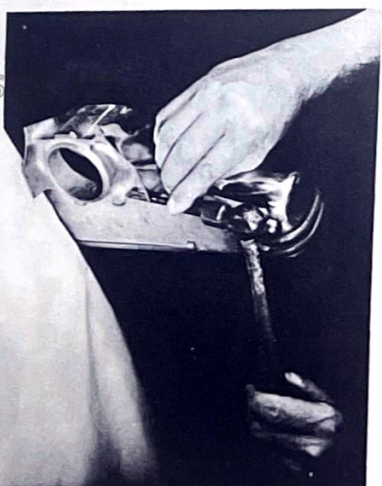
Figure 2-5. Tap casting as indicated to tighten or level
