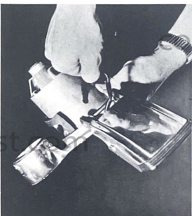
Figure 1-51. Removing headlight wires from motor housing.
