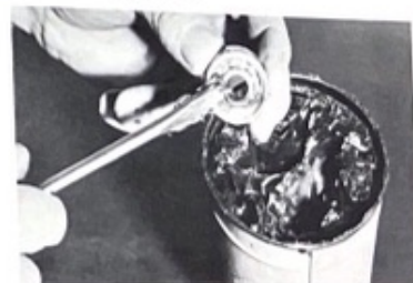
Bearing can be pushed out of plate by using thumb pressure only.
