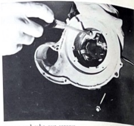
Loosen the two lock nuts on field core mounting screws and take out screws.
