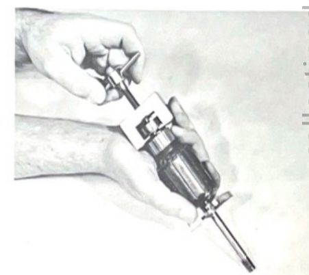
Figure 1-16. Removing rear bearing from armature
