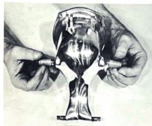
Figure 1-22. Installing brush holders in motor housing
