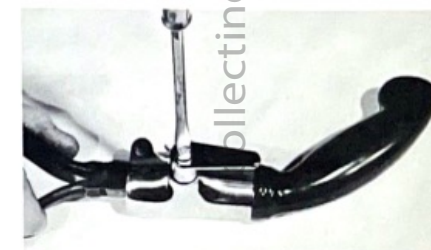
Figure 3-2. Removing cord swivel hook
